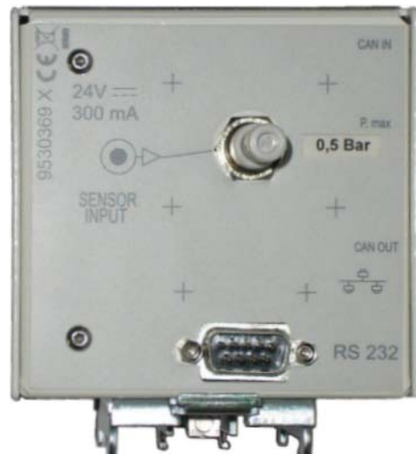
Test pressure supply side.
