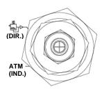
Instant fitting: 8, 10 or 12 mm diameter for 1 MPa range maximum.
