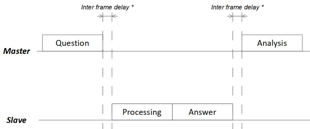
\* 3,5 times the transmission time of a byte
