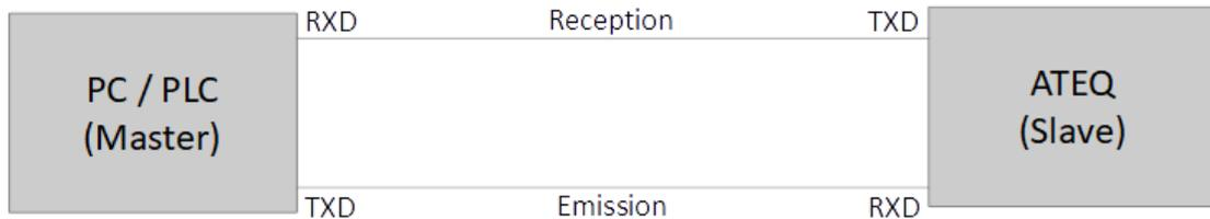
The network is built on the basis of a cable composed of two pairs of entwined and shielded wires. One pair is for the signals and the other is for the ground.
