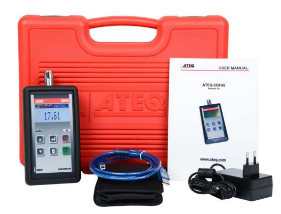
Carrying case Protective holster and soft case USB cable: To connect the instrument to a PC. **Power supply:** The power supply of the CDP60 converts a network voltage (120 to 240 V AC) into a 24 V DC low voltage supply
